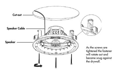
Center the speaker in the cutout. Rotate the frame as needed before tightening the screws. Tighten the screws equally until the clamps secure the frame. **Do not overtighten.**
